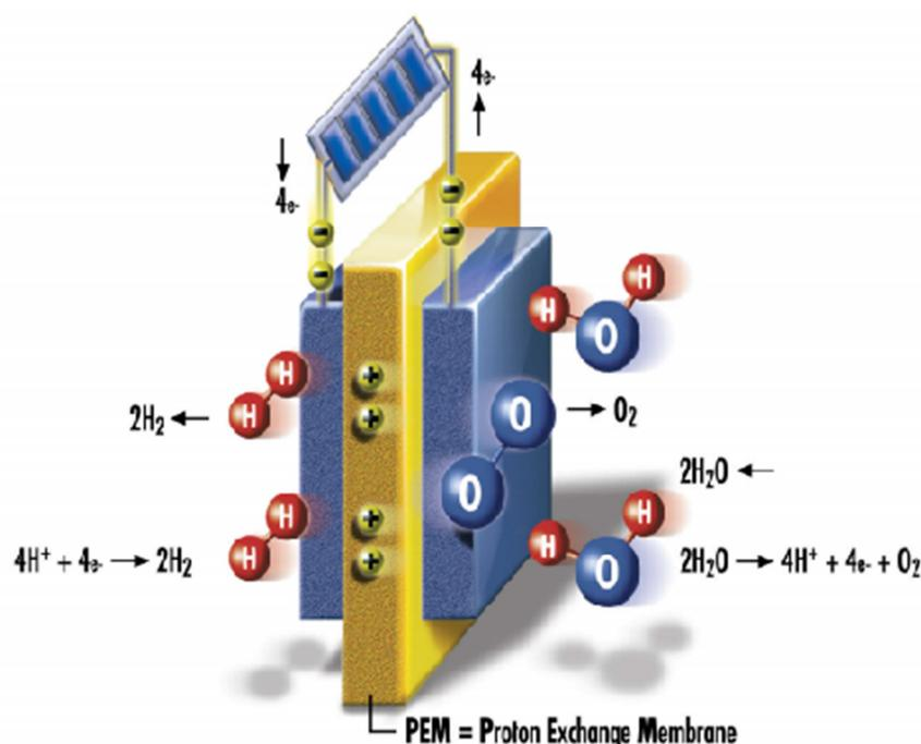
Fig. 1 Scheme of a PEM electrolyser.
