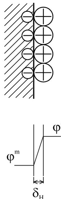
**Figure 2 :** Helmholtz model of the electrode double layer and development of potentials in it.
